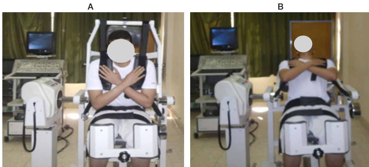
Figure 3. Starting (A) and ending (B) position for measurement of muscle peak torque
